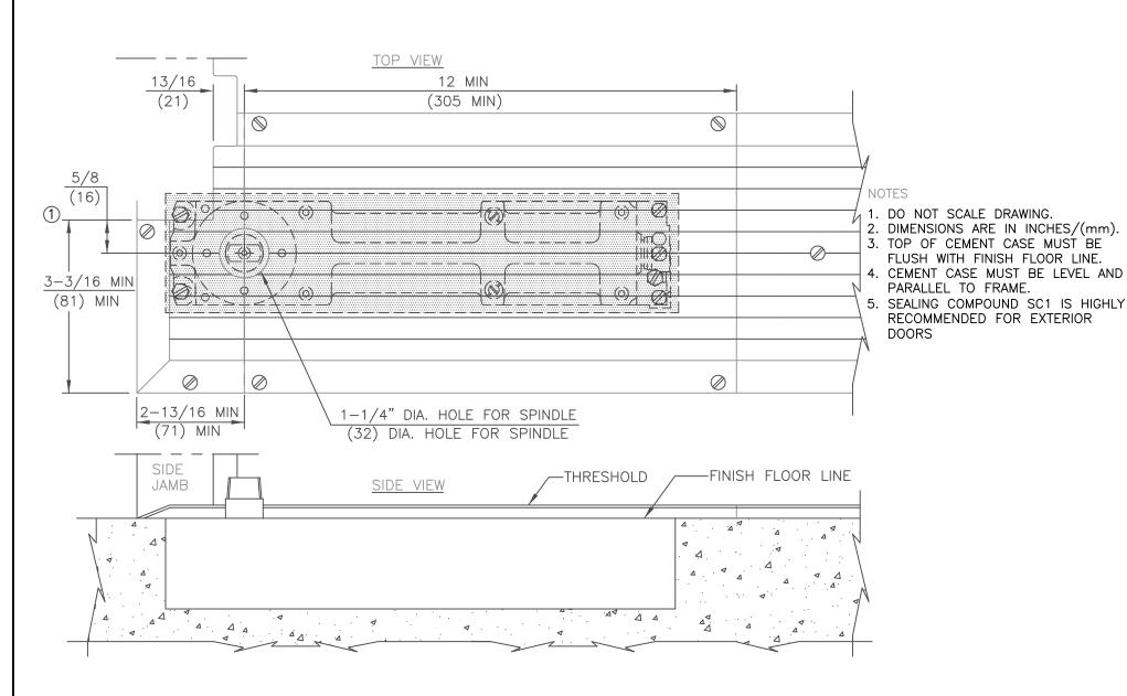
THRESHOLDS IN CONJUNCTION WITH BTS SERIES 3/4" OFFSET FLOOR CLOSER
